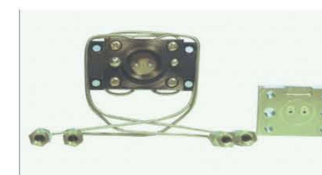
The heart of UV detector: flow cell
